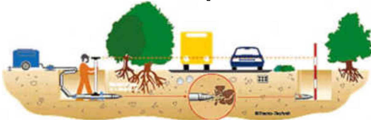
Figure 3.20 Representative Image of Trenchless Technology and Components for Installation of Underground Cables
